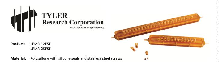
The LPMR-12PSF and LPMR-25PSF are manufactured from polysulfone, an advanced engineered thermoplastic polymer capable of withstanding a temperature range of -100°C to 150°C. The LPMR-PSF series biofilm devices may be safely sterilized using an autoclave provided instructions are followed carefully.
